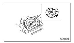
Remove the jack, necessary tools, spacers and spare wheel from the luggage compartment.
