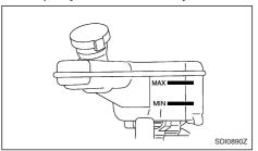
Check the fluid level in the reservoir. If the brake fluid is below the MIN line, the brake warning light comes on. Add fluid up to the MAX line. See "Ca-
