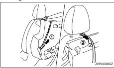
1. Remove the hook (1) from the anchor on the underside of the cushion.
