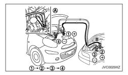
1. Prepare vehicle (A) with the booster battery for the vehicle (B) being jump-started.
