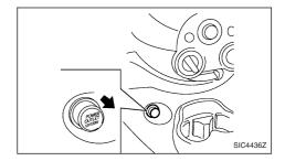
The power outlet is for powering electrical accessories such as mobile telephone.
