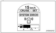
If the [SYSTEM ERROR] display appears and/or the ON indicator light on the parking space measurement switch blinks, have the system checked by a NISSAN dealer or qualified workshop.
