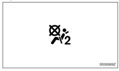
When the ignition switch is in the "ON" position, the front passenger air bag status light on the meter illuminates for about 7 seconds and then turns off. This indicates that the front passenger air bag system is operational.
