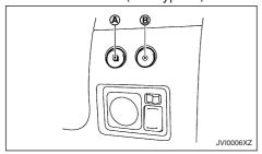
Switches for the trip computer are located on the left or right side of the combination meter panel. To operate the trip computer, push the switches as shown above.
