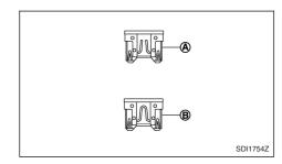
6. If the fuse is open (A), replace it with a new fuse
