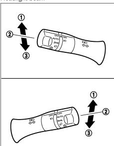
To turn on the high beam, push the lever towards the front position (1).
