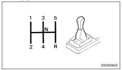
To change gears, or when upshifting or downshifting, fully depress the clutch pedal, shift into the appropriate gear, then slowly and smoothly release the clutch pedal.
