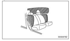
The supplemental side-impact air bag is located at the outside of the front seats' seatbacks.
