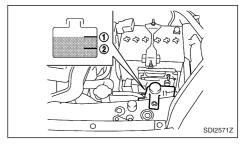
Check the coolant level in the reservoir when the engine is cold. If the coolant level is below MIN level (2), add coolant up to the MAX level (1). If the reservoir is empty, check the coolant level in the radiator when the engine is cold. If there is insufficient coolant in the radiator, fill the radiator with coolant up to the filler opening and also add it to the reservoir up to the MAX level (1).
