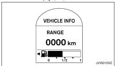
The distance to empty (dte) mode provides you with an estimation of the distance that can be driven before refuelling. The dte is constantly being calculated, based on the amount of fuel in the fuel tank and the actual fuel consumption.
