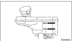
Check the fluid level in the reservoir. If the fluid is below the MIN line. Add fluid up to the MAX line. See "Capacities and recommended fuel/lubricants" in the "9. Technical information" section for the recommended fluid type.
