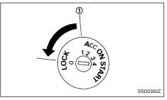
The ignition lock is designed so that the ignition switch cannot be turned to the "LOCK" position until the selector lever is moved to the P (Park) position. When moving the ignition switch to the "LOCK" position, to remove the key from the ignition switch, make sure the selector lever is in the P (Park) position.
