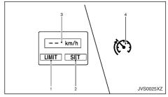
The speed limiter operating condition is shown on the vehicle information display and instrument panel.
