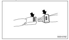
The centre seat belt buckle and the tongue are identified by the CENTER mark. The centre seat belt tongue can be fastened only into the centre seat belt buckle.
