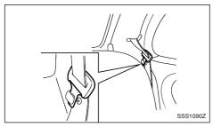
Hook the seat belt at the belt hook when folding down the rear seat.
