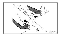
2. Adjust the seat belt length. To shorten, hold the tongue and pull the upper belt as illustrated (1). To lengthen, hold the tongue and pull the under belt as illustrated (2).
