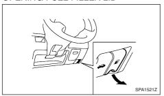
To open the fuel filler lid, pull the fuel filler lid release handle.
