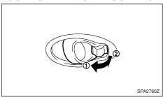
To lock the front doors, push the inside lock knob to the lock position (1), and then close the door while pulling the door handle.
