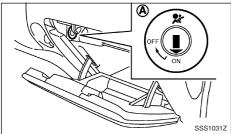
The front passenger air bag can be turned off with the front passenger air bag switch (A) located inside of the glove box.
