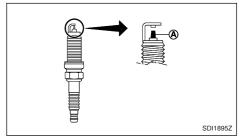
It is not necessary to replace the iridium-tipped (A) spark plugs as frequently as the conventional type of spark plugs. These spark plugs are designed to last much longer than the conventional type of spark pluq.
