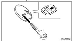
To remove the mechanical key, release the lock knob at the back of the Intelligent Key.
