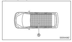
The Intelligent Key can only be used for starting the engine when the Intelligent Key is within the specified operating range (1).
