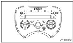
The audio system operates when the ignition switch is in the "ACC" or "ON" position.
