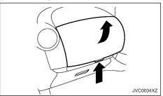
To open the upper instrument box, push the button.
