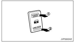
Power door lock switch (located on the centre console)
