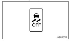
The vehicle should be driven with the Electronic Stability Programme (ESP) system on for most driving conditions.
