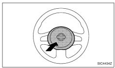
The horn switch operates with the ignition switch in any position except when the battery is discharged.
