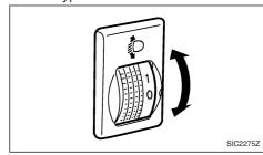
The headlight aiming control operates when the ignition switch is in the "ON" position and the headlight is on to allow the headlight axis to be adjusted according to the driving condition.
