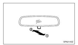
Pull the adjusting lever (1) (where fitted) when the glare from the headlights of the vehicle behind you obstructs your vision at night.
