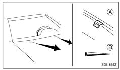
Be careful not to clog the washer nozzle (A). This may cause improper windscreen washer operation. If the nozzle is clogged, remove any objects with a needle or small pin (B). Be careful not to damage the nozzle.
