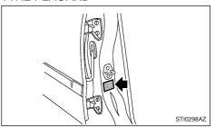
The cold tyre pressures are shown on the tyre placard fixed to the side of the driver's side centre pillar.
