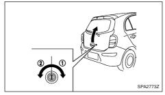
To lock the back door, push it down firmly, insert the key to the door key cylinder and turn the key clockwise (1). To unlock the back door, turn the key anticlockwise (2).
