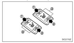
The seats can be warmed by built-in heaters. The switches located on the centre console can be operated independently of each other.
