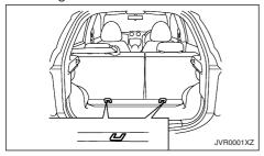
The anchor points are located on the seat cushion behind the rear seats outboard seating positions.
