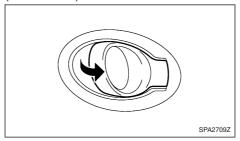
To unlock and open the door, pull the inside door handle as illustrated.
