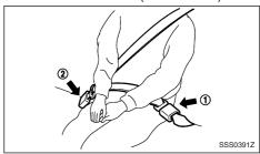
The rear centre seat belt has a connector tongue ① and a seat belt tongue ②. Both the connector tongue and the seat belt tongue must be securely latched for proper seat belt operation.
