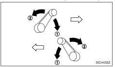
The side windows can be opened (1) or closed (2) by turning the hand crank on each door.
