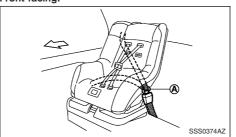
If you must install a front-facing child restraint system on the rear seat, follow these steps:
