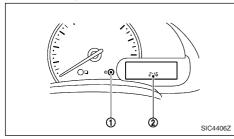
The digital clock (2) in the meter displays the time when the ignition switch is in the "ON" position.
