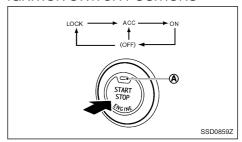
When the ignition switch is pushed without depressing the brake pedal (Continuously Variable Transmission models) or the clutch pedal (Manual Transmission models), the ignition switch position will change as follows:
