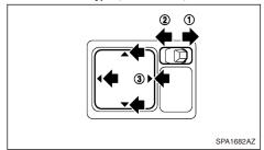
The outside rearview mirror remote control operates when the ignition switch is in the "ACC" or "ON" position.
