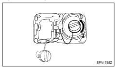
The fuel filler cap is a ratcheting type. Turn the cap anticlockwise (1) to remove. Tighten the cap clockwise (2) until ratchet clicks, more than twice, after refuelling.
