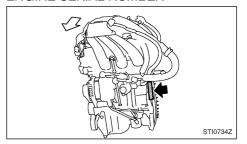
The number is stamped on the engine as shown.
