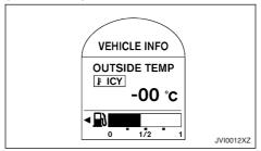
The outside air temperature is displayed in °C in the range of -30 to 60°C.
