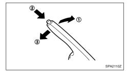
To apply the parking brake, pull the parking brake lever up (1).
