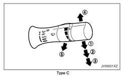
The windscreen wiper and washer operate when the ignition switch is in the "ON" position.
