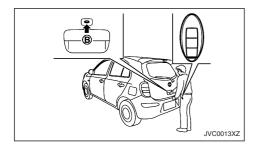
When you carry the Intelligent Key with you, you can lock or unlock all doors by pushing the door handle
