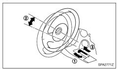
While pushing the lock lever down (1), adjust the steering wheel up or down (2) until the desired position is achieved.
