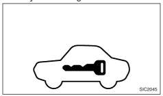
The security indicator light is located on the meter panel. It indicates the status of NATS.
