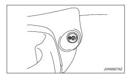
The USB/AUX connector is on the lower centre of the instrument panel.
