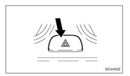
The hazard indicator flasher switch operates with the ignition switch in any position except when the battery is discharged.
