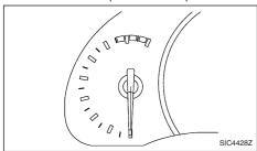
The tachometer indicates the engine speed in revolutions per minute (rpm).
