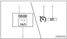
The cruise control operating condition is shown on the vehicle information display and instrument panel.
