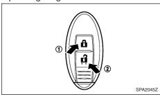
It is possible to lock/unlock all doors including the back door using the remote keyless entry system. The operating distance depends upon the conditions around the vehicle. To securely operate the lock and unlock buttons, approach the vehicle to about 1 m (3.3 ft) from the door.
